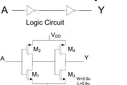
Circuit Schematic (Including Device Sizing)
