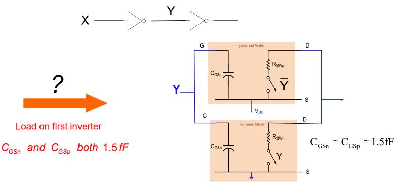
Loading effects same whether  $C_{GSp}$  and/or  $C_{GSn}$  connected to  $V_{DD}$  or GND
