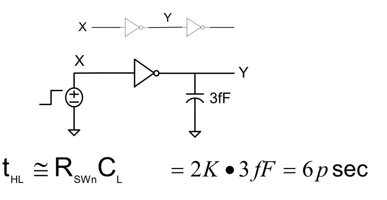
$$\mathbf{t}_{\text{\tiny LH}} \cong \mathbf{R}_{\text{\tiny SWp}} \mathbf{C}_{\text{\tiny L}} = 6K \bullet 3 fF = 18 p \sec \mathbf{C}$$
