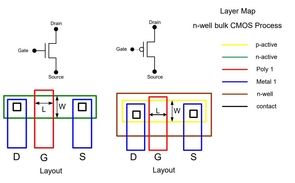
Layout always represented in a top view in two dimensions
