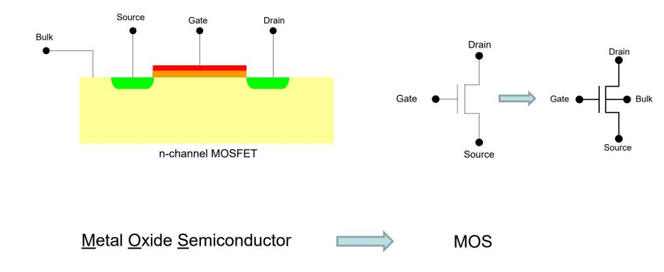
Early processes used metal for the gate, today metal is seldom used but the term MOS transistor is standard even though the gate is no longer metal
